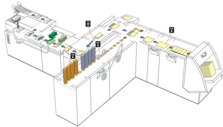
**Pace connected to an inserting system** offers a flexible solution for producing ready-to-mail envelopes. The number of enclosure feeders can be freely selected, guaranteeing the necessary flexibility for individualized compilation of mailpieces. A wide range of post-processing options is also available for this configuration.
