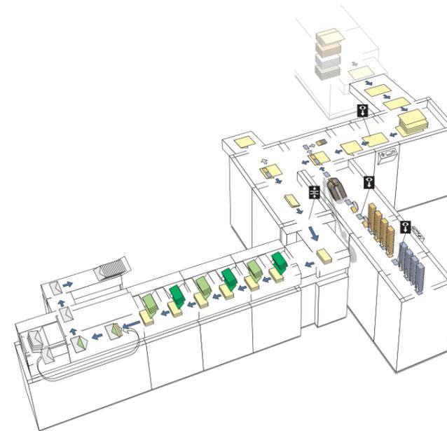
The **integrated self-mailer Flexi Card**, enables Pace to prepare printed documents for mailing without inserting. With speeds of up to 8,000 sheets per hour, the high-capacity self-mailer safely folds and seals documents using heat and pressure. A clean, reliable and economical solution for creating cost-effective mailings.
